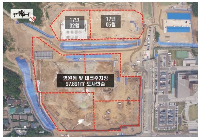
[Estimation of earth volume using GPS coordinates from a drone]
